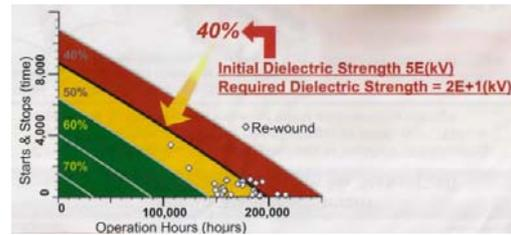
Gambar 18 Batas Maksimal Residual Breakdown Voltage
