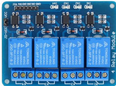
Gambar 2. 2 Module relay 4 channel
