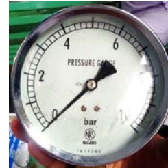
Gambar 14: Pressure Gauge Nagano 0-10 bar
