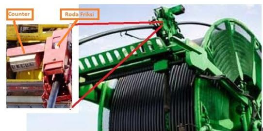
Gambar 1. Coiled Tubing Depth Counter
