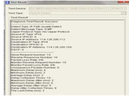
Gambar 4.1. Hasil Test Ping RNC ke interface secondary link
