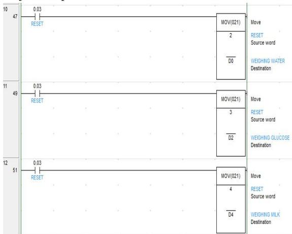
Gambar 4.24 Ladder reset water, glucose, milk
