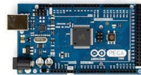
Gambar 1.2 Arduino Mega 2560
