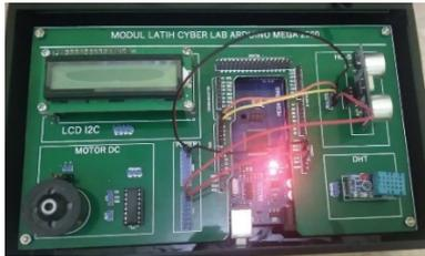
Gambar 5. Instalasi sensor ultrasonik HC-SR04
