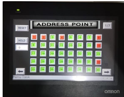
Figure.23 Mapping Address Point E. Digital Direct Bit – Output PLC
