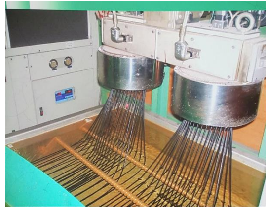
Fig. 3c Fibre Drawing Process
