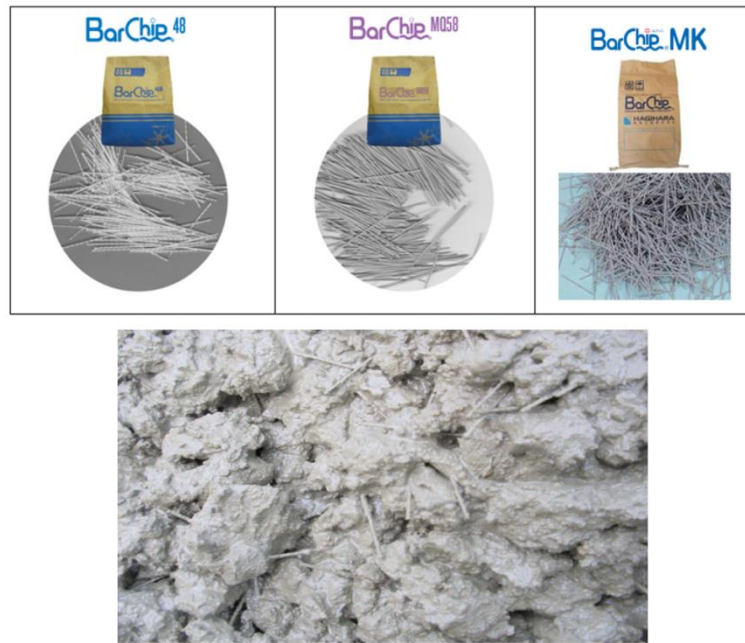
Fig 1. Various forms of Polypropylene Fiber (Barchip) and mixed with concrete Source: www.barchips.com
