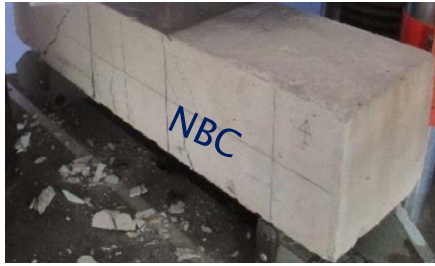
Fig. 9 Crack pattern of NBC-2
