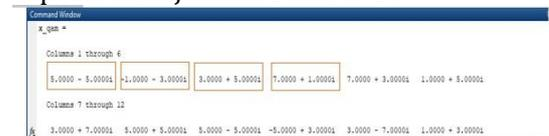
**Gambar 8.** Hasil Konversi Bit to Simbol 64 QAM
