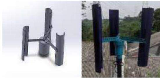
**Gambar 11.** Detail Gambar Small turbin angin tipe vertikal
