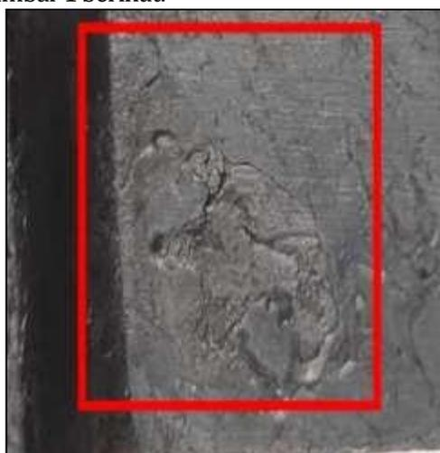
**Gambar 1.** Cacat *Flowline* Pada Part
