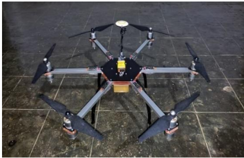
Gambar 2. Frame Double Hexacopter
