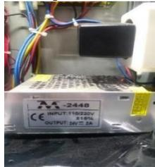
**Gambar 3.** Power Supply 24V 2A
