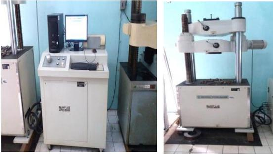
**Gambar 1.** Alat uji tarik Testing Machine 100 T, GT7001 – LG, SN : TC 08 01 393, Cap : 1 Ton di BLK Condet
