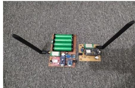
Gambar 25 Transmitter dan Receiver
