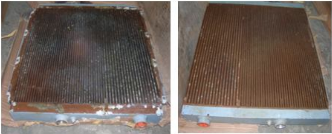
Figure 1. The as received failed compressor after-cooler that was used for the present study
