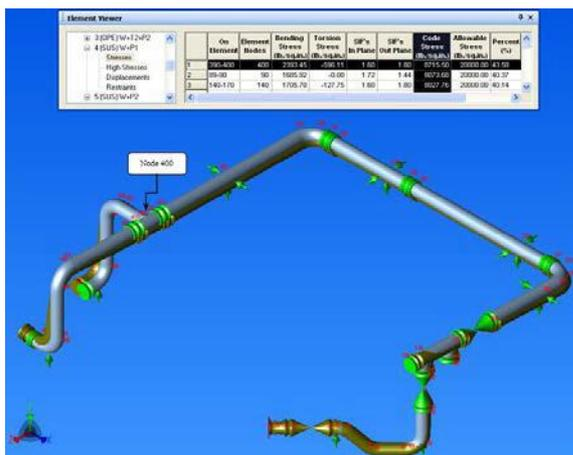
Gambar 4.1. Permodelan tegangan pipa akibat Beban Sustain
