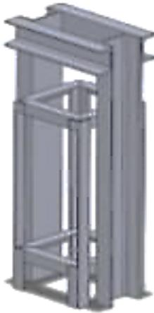
Gambar 6. Rangka Mesin Press Geram
