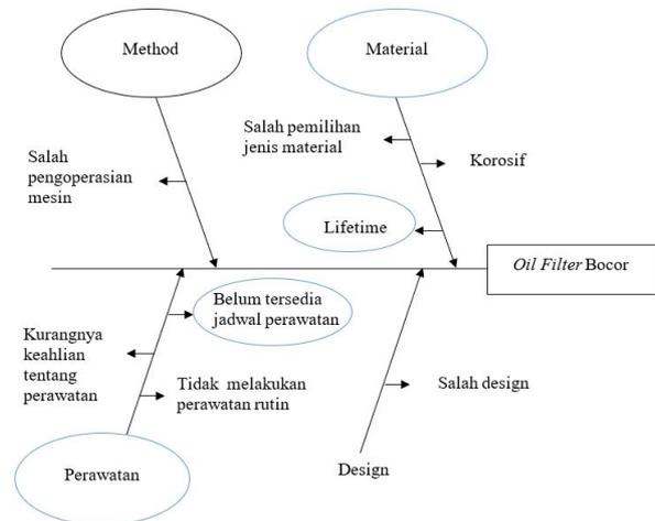
Gambar 4. Fishbone Diagram
