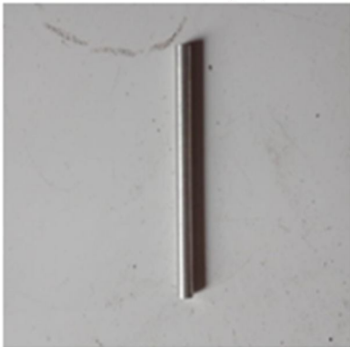
Gambar 3.3 Material Alat Uji Logam Alumunium 6061 (Al)
