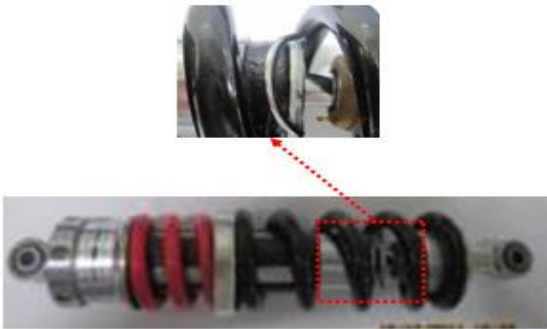
Gambar 3. Crack Area Rolling Damper
