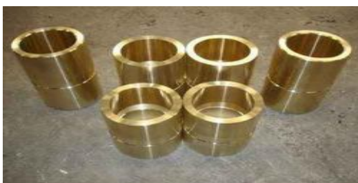
Gambar 1 Potongan Seating Klep Alumunium bronze AB2
