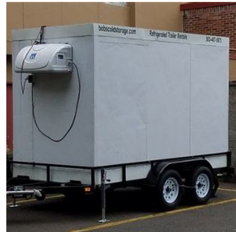
Gambar 2. 3 Mobile Cold Storage (sumber: www.bobscoldstorage.com )
